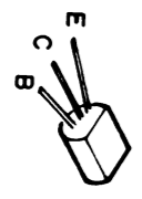
O102 ~ O105 2SC461 (C) O106, 715, 716, 901, 902 O501 ~ 510 2SC1775AV (F) O302, 306, 307, O409, 410, 771 ~ 774, O802, 832 2SC945A (P, Q) O303 ~ 305, 407, 408, 411 O719, 720 2SA733A (P, Q) O821 2SD438
